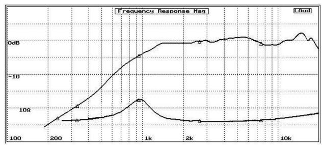
Anechoic 2pi Frequency Response Curves on axis, and impedance
