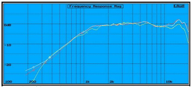
North D25-06S Frequency Response 0 degrees, 5 degrees and 15 degrees (anechoic 1 meter)
